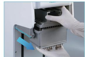
Pull out the pipetting head
